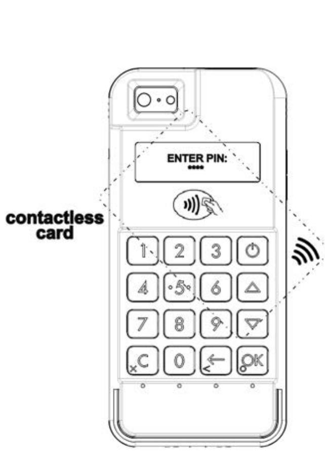
**Figure 8: Contactless Card (RFID) Reader**
